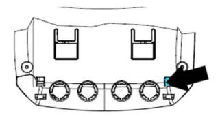
Leave a gap at least 0.8 cm wide between the sensor and installation wall. Do not place the sensor near objects that could heat and alter temperature readings.
